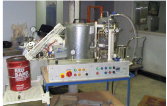
Figure 2 Foamed bitumen testing device
